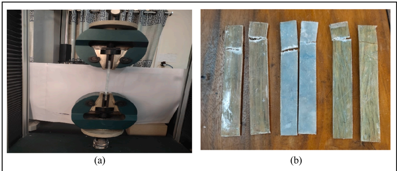
Fig. 3. Fig. of UTM tensile testing machine and broken tensile test sample (a) UTM machine, (b) Tensile test sample.
